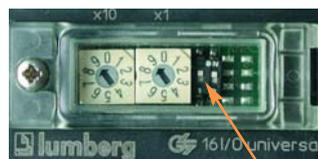
The undervoltage diagnostics of the actuator system power supply can be switched off with the left DIP switch.
