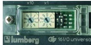
The valid address range lies between 0 and 63. The address is set to 63 when switched to a value in the range of 64 to 98. The factory setting for the address is 63.
