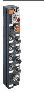
8 IN/8 OUT universalLioN-Link I/O module with 8 digital I/O channels, channels can be used universally as inputs or outputs, M8 sockets (8x), 3 poles, M12 actuator supply
