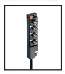
The LioN-Link 0941 UNC 601/...M power module is used for decentralized power supply for I/O modules. It has four ports, two potential circuits and a 10 m lead with a conductor gauge of 5x1 mm². This provides for bridging distances of up to 25 m without voltage loss as well as for configuring separate potential groups each with their own fuses.
