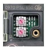
The adjustable address range lies between 1 and 99. The factory setting for the address is 99.
