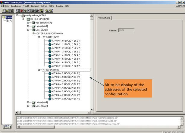
The 0970 PSL 650 module can be used as a simple input/output module as well as a mixed input/output module. You do not have to configure the I/O any further when using it as a universal module. Each channel can be used as an input or as an output.
